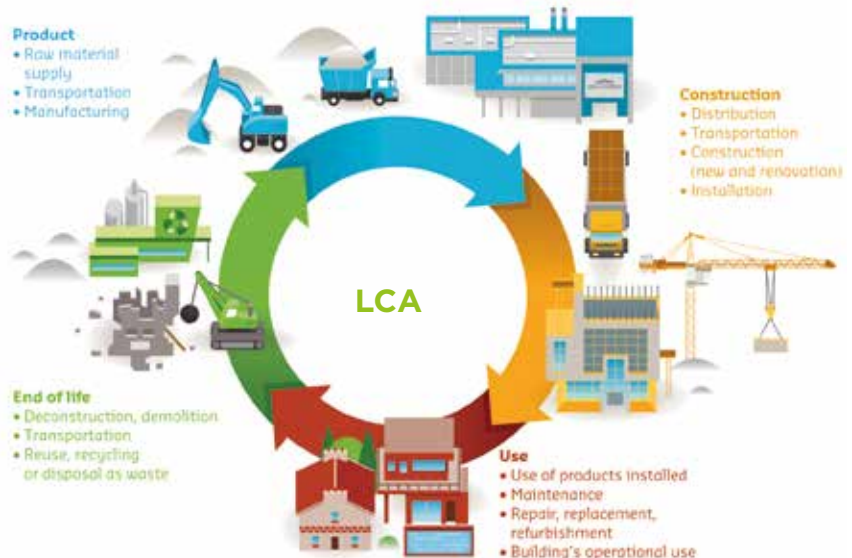
Life Cycle Assessment of a construction product
