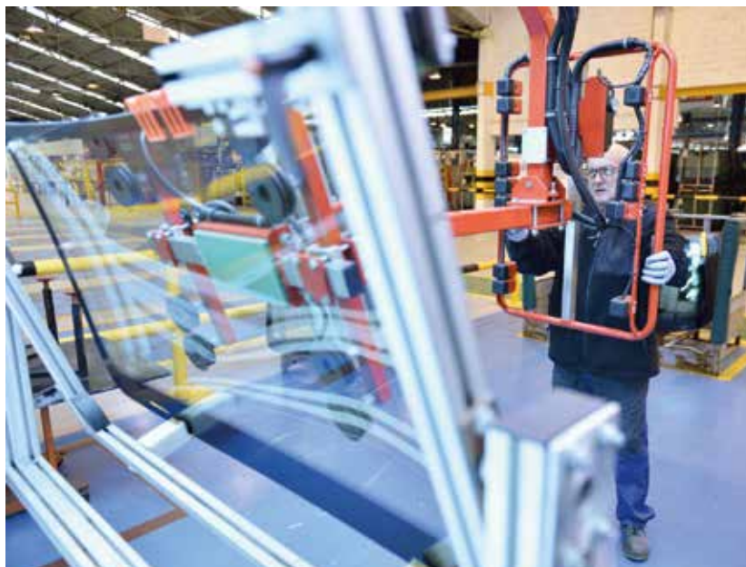
Handling assistance system at Saint-Gobain Sekurit in Avilès (Spain)
